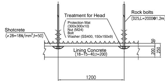
Figure 10.5. Standard cross-sectional view (left) and support pattern (right) of class CII.
