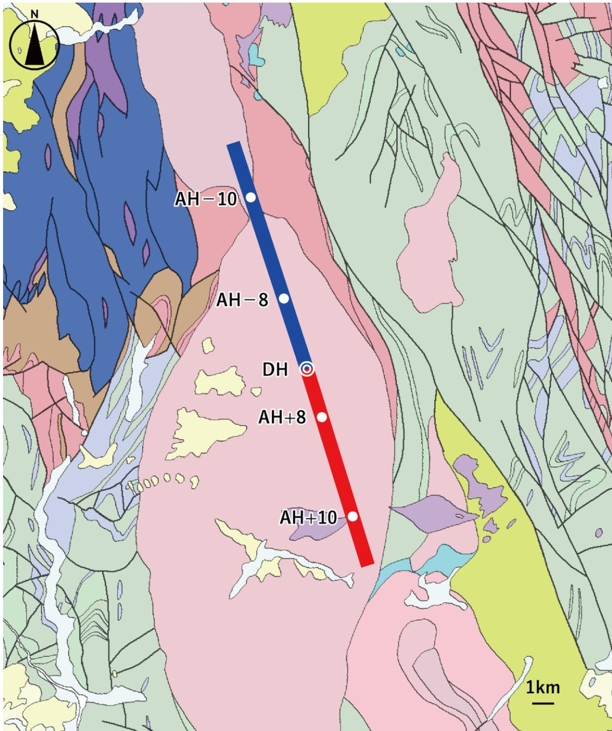
Figure 6.2. A plan view of the geology of the ILC facility location plan (blue line: the main linear accelerator for electrons (a length of 10.9 km), red line: the main linear accelerator for positrons (a length of 9.6 km)).
