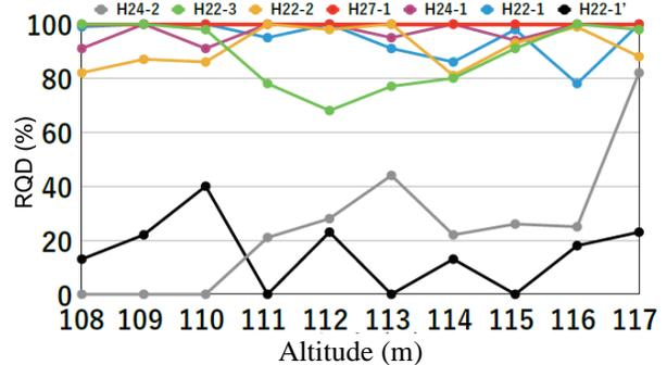
Figure 4.3. Pictures and the RQD of the cores near an altitude of 110 m (the numbers added to the core pictures indicate depths (m)).
