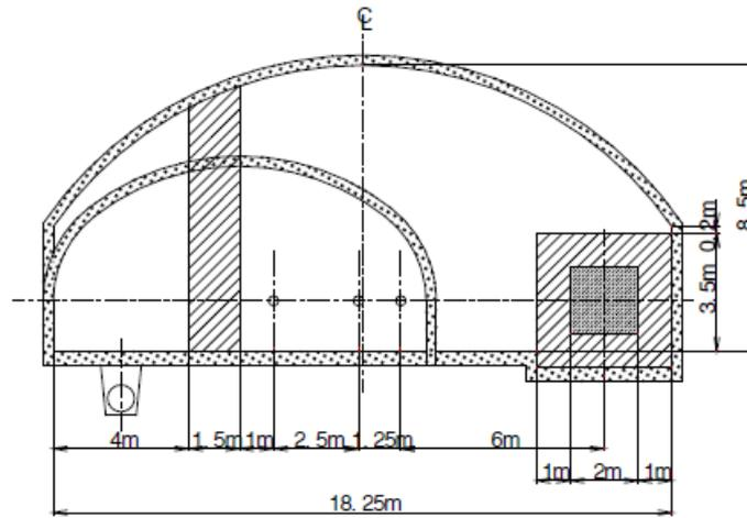
Figure B.4. Cross section C-C of the main beam dump cavern.
