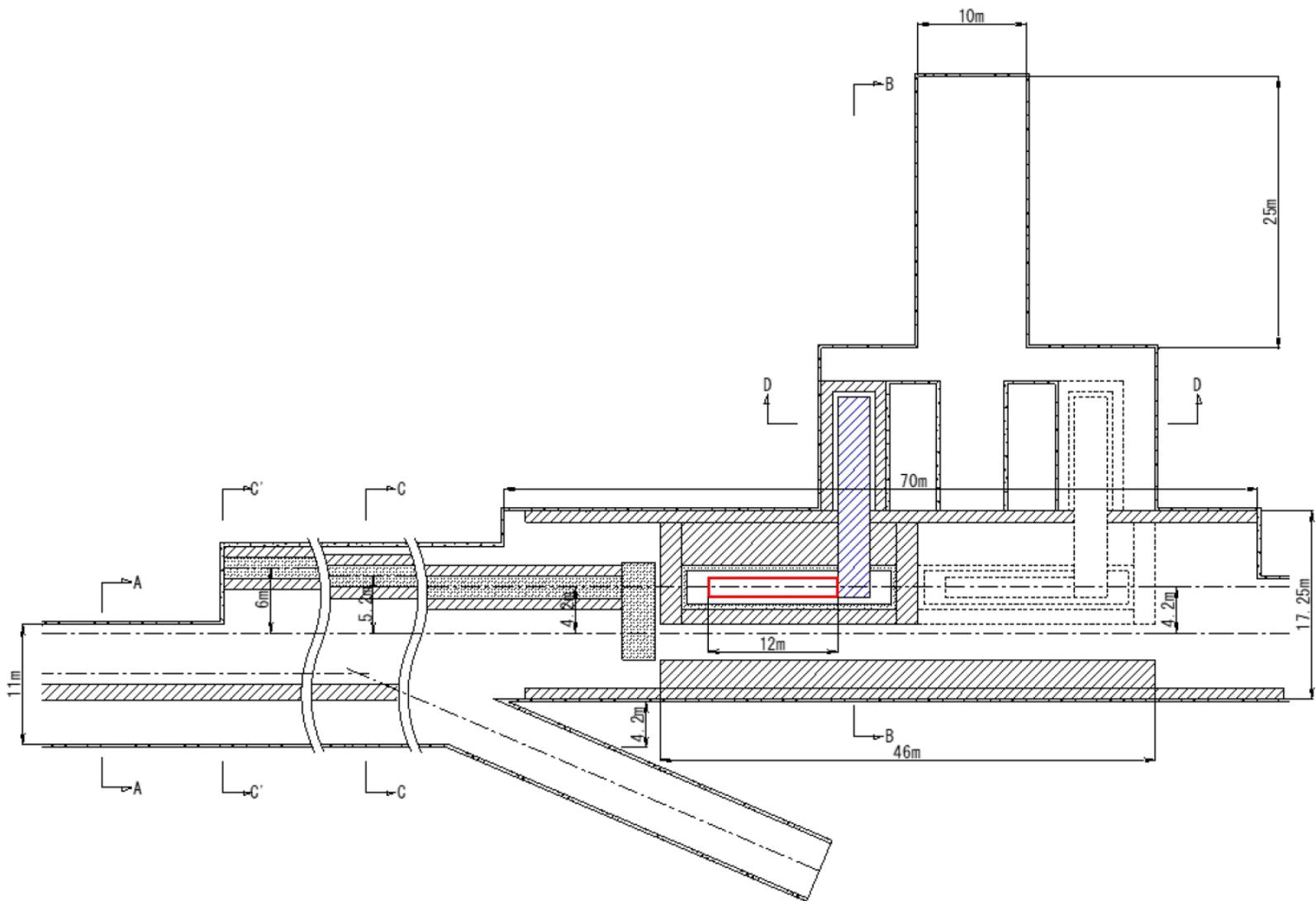
Figure B.1. Plan view of the periphery of the main beam dump cavern.
