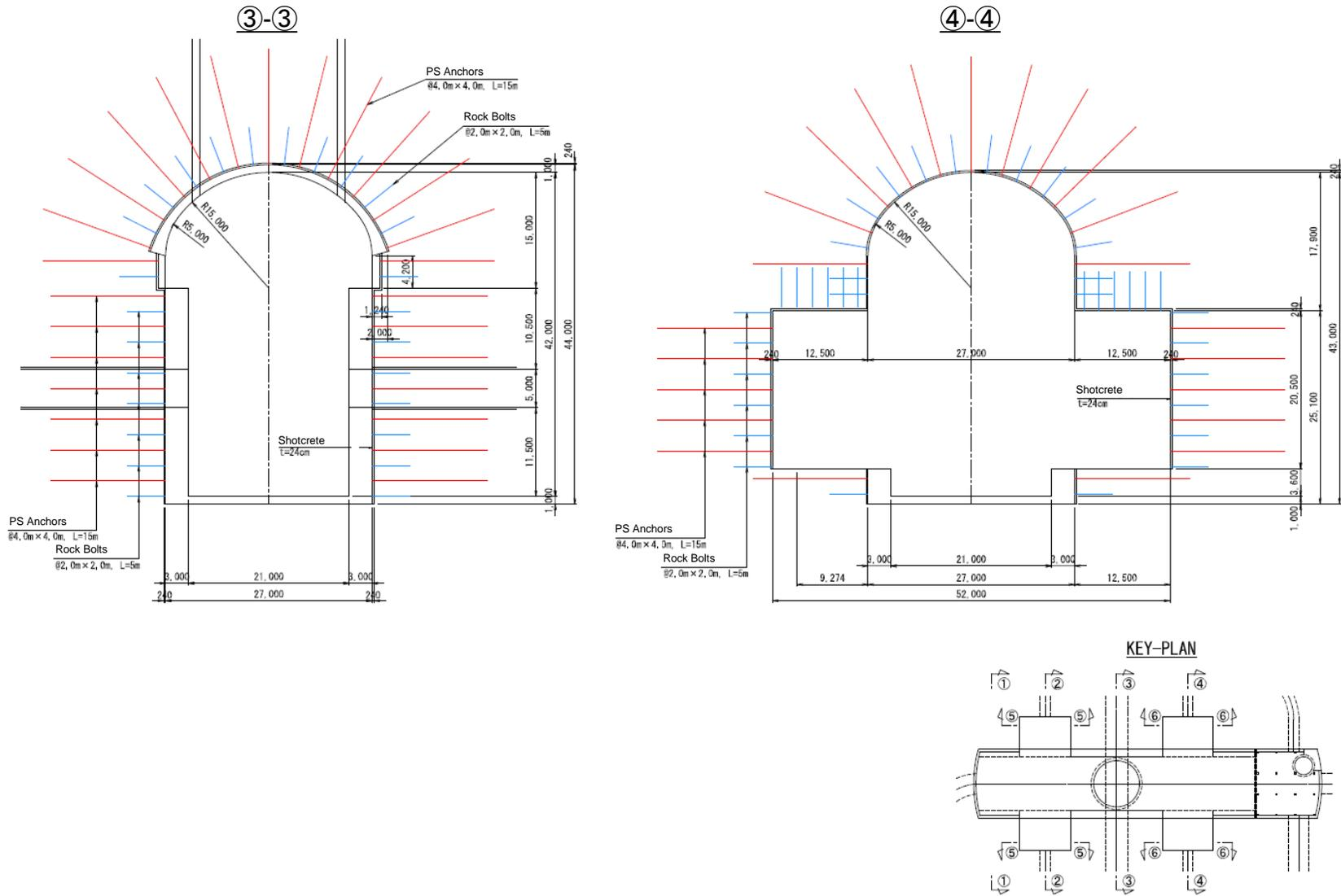
Figure 9.3. Standard support pattern (2) of the detector hall.
