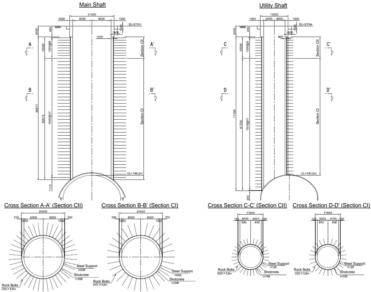
Figure 9.5. Standard support patterns of the main shaft and utility shaft.
