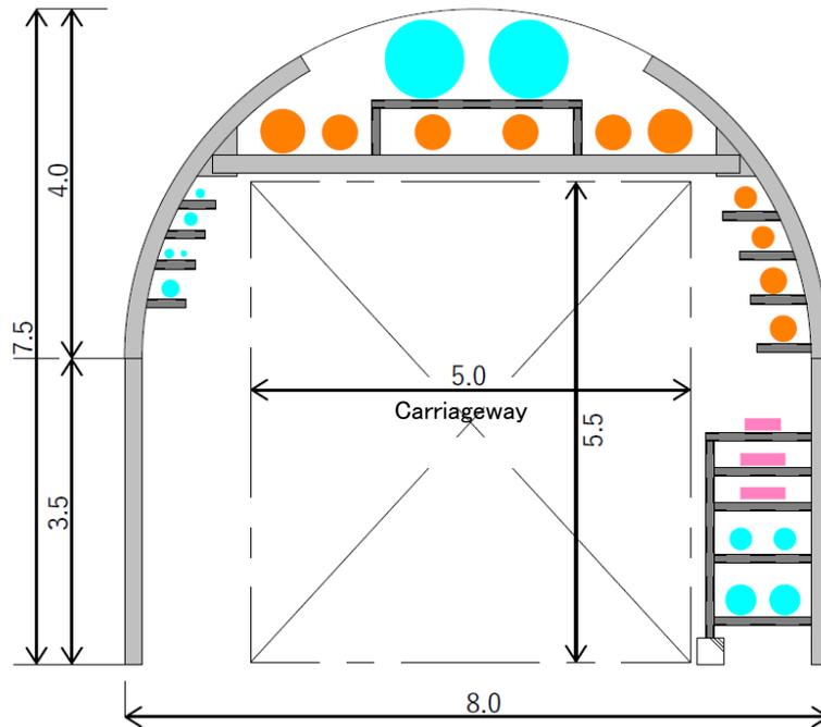
Figure 2.2. A plan of piping and cabling in the access tunnel (under consideration).
