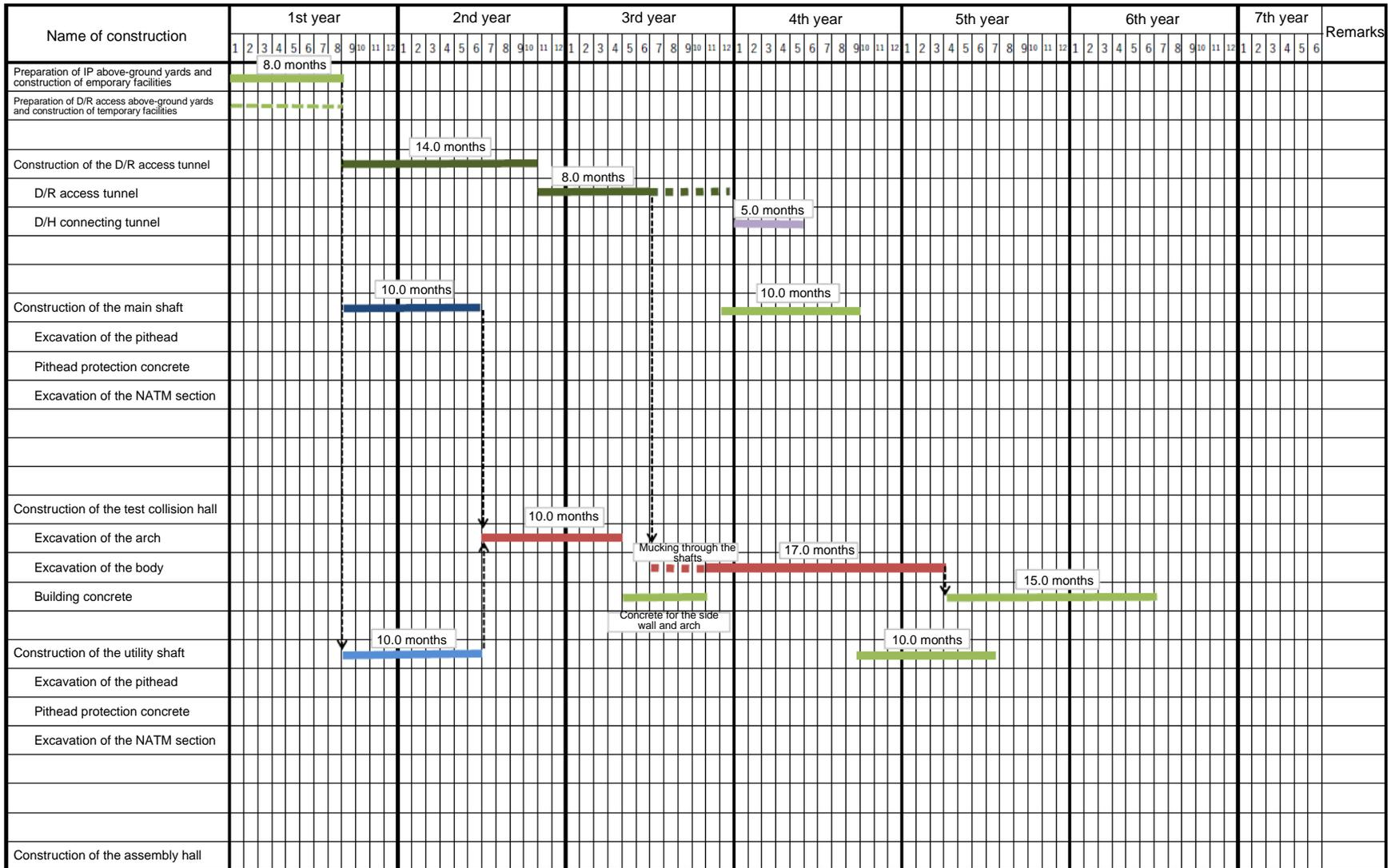
Figure 9.7. Processes for the detector hall, shafts, and peripheral tunnels
