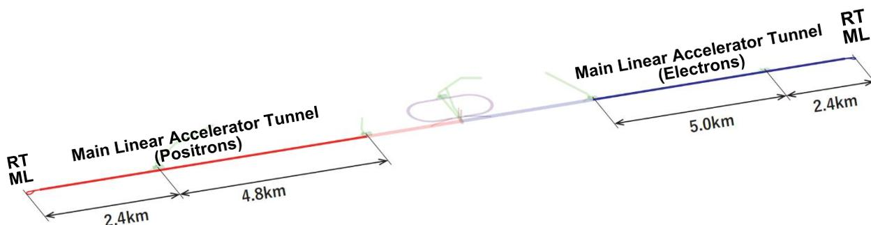
Figure 2.7. Main linear accelerator tunnels.
