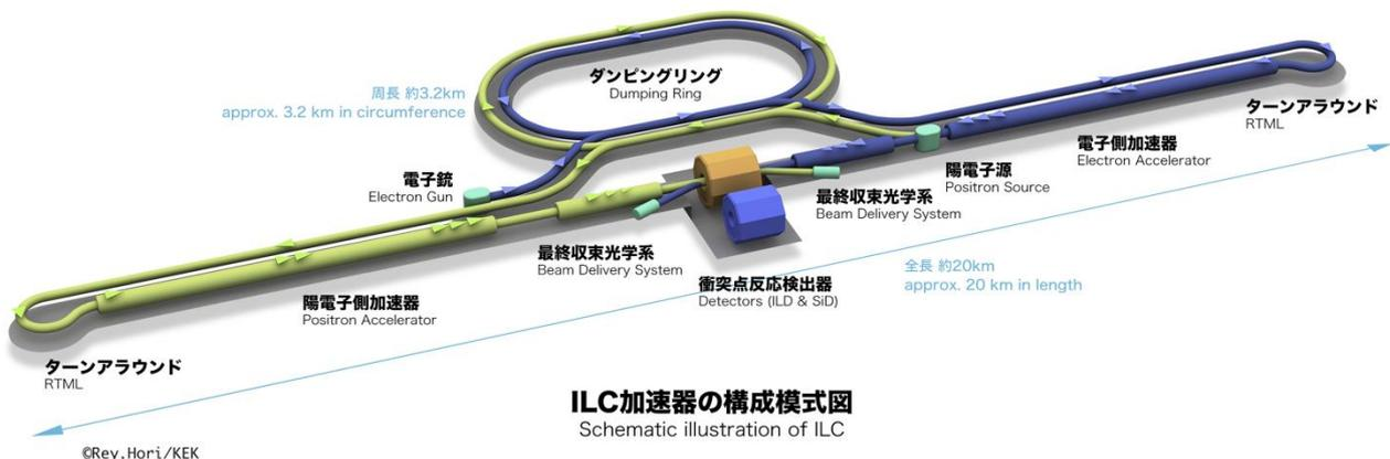
Figure 1.1. Configuration of the ILC accelerator.
