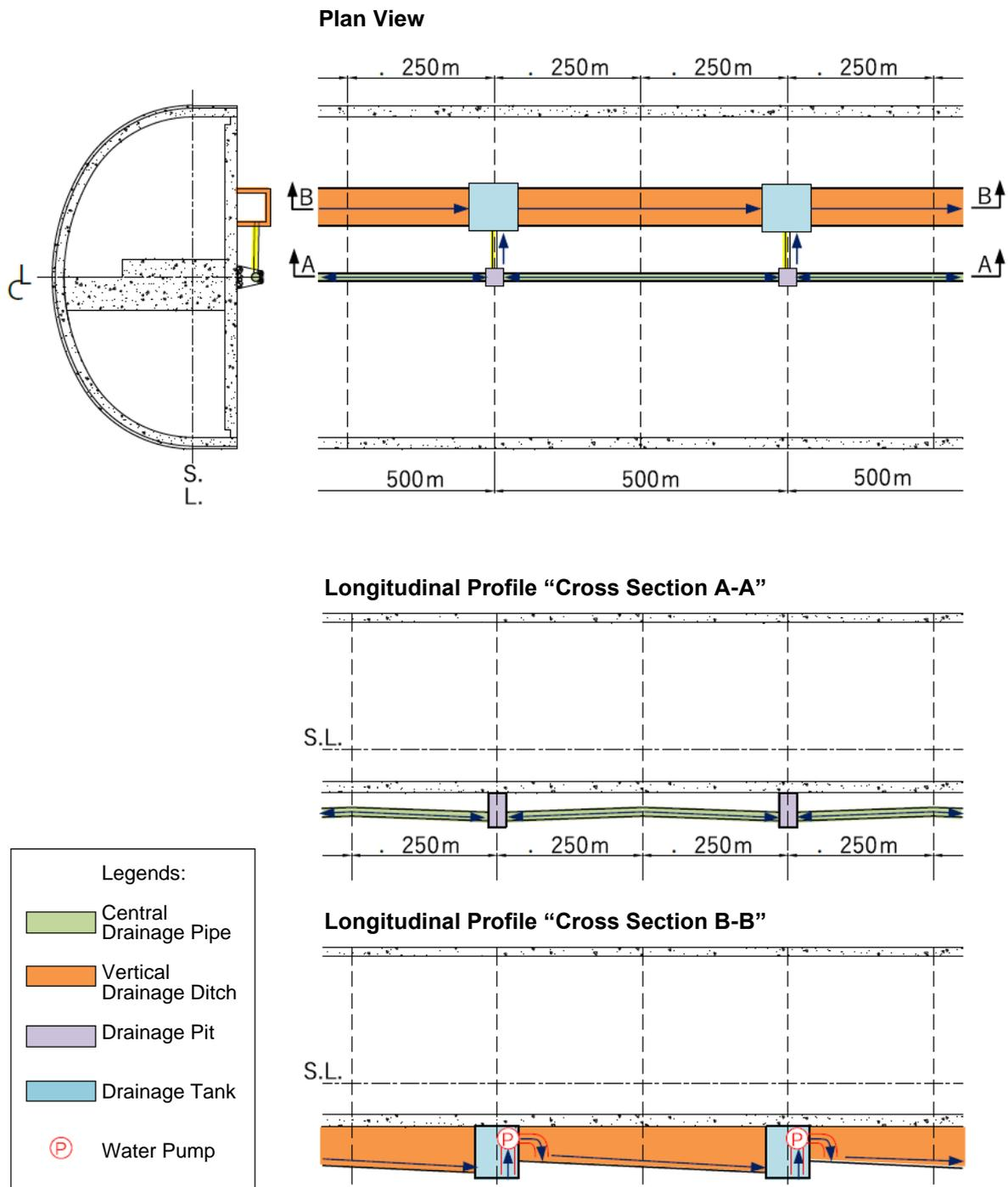
Figure 10.2. A schematic drawing of the sectional drainage system in the accelerator tunnel.
