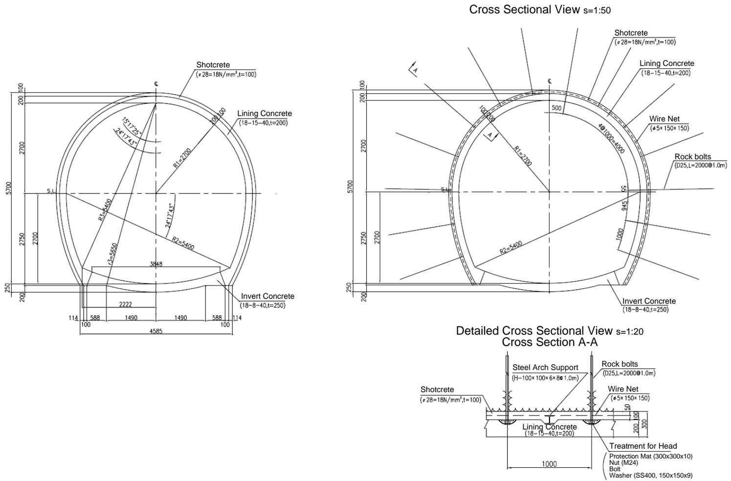
Figure 10.6. Standard cross-sectional view (left) and support pattern (right) of class DI.
