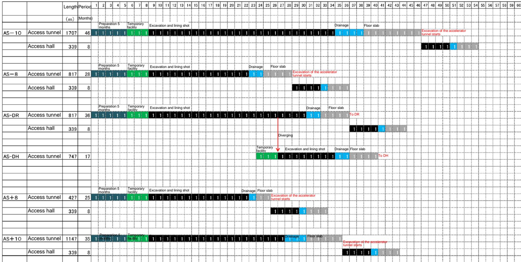
Figure 7.11. Processes for the access tunnels and access halls.
