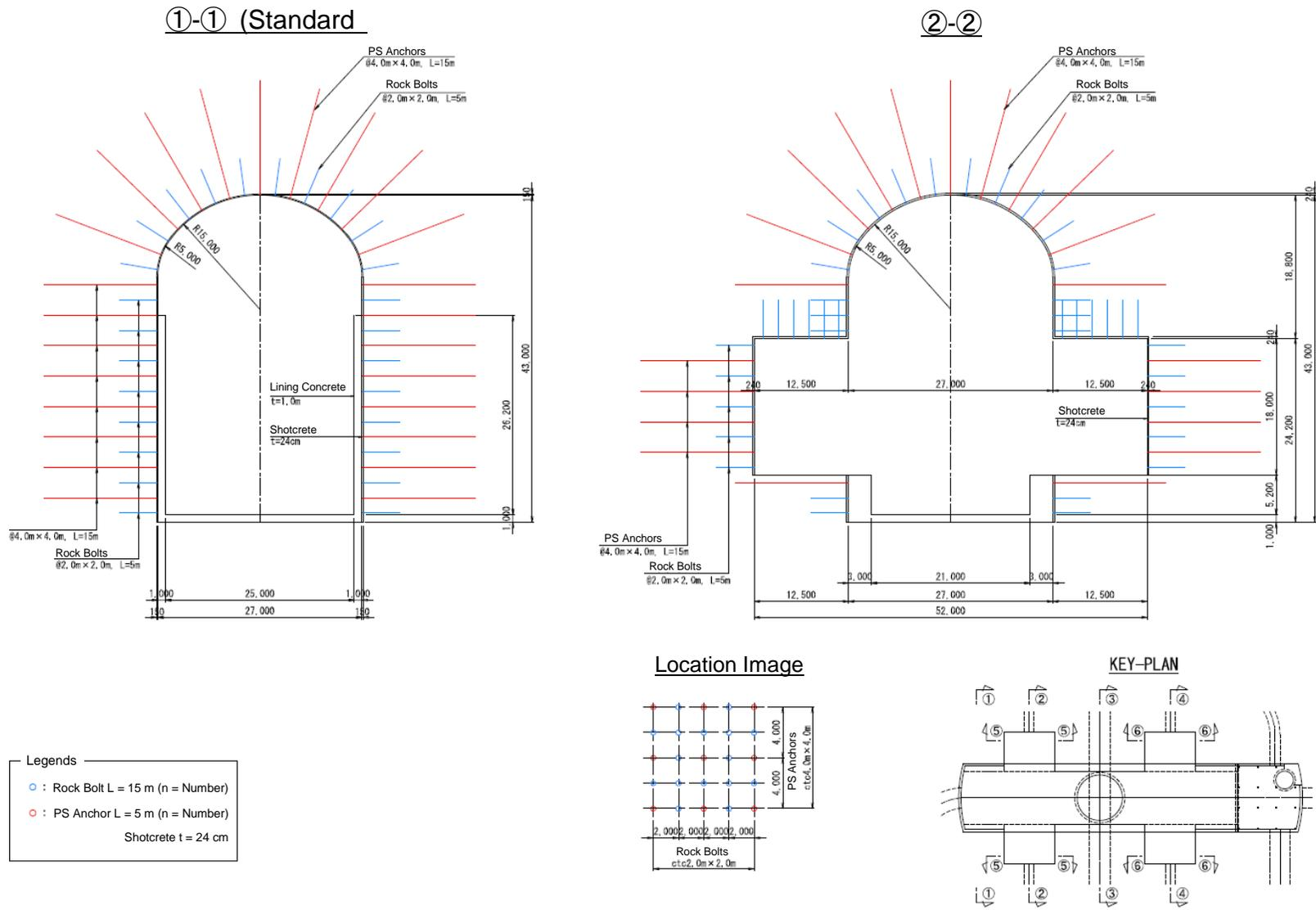
Figure 9.2. Standard support pattern (1) of the detector hall.
