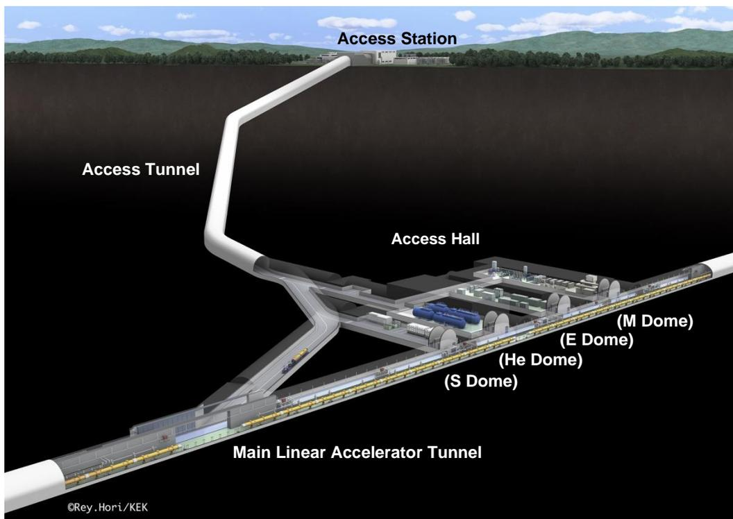
Figure 2.3. An illustration of a connection from an access station to a main linear accelerator tunnel.
