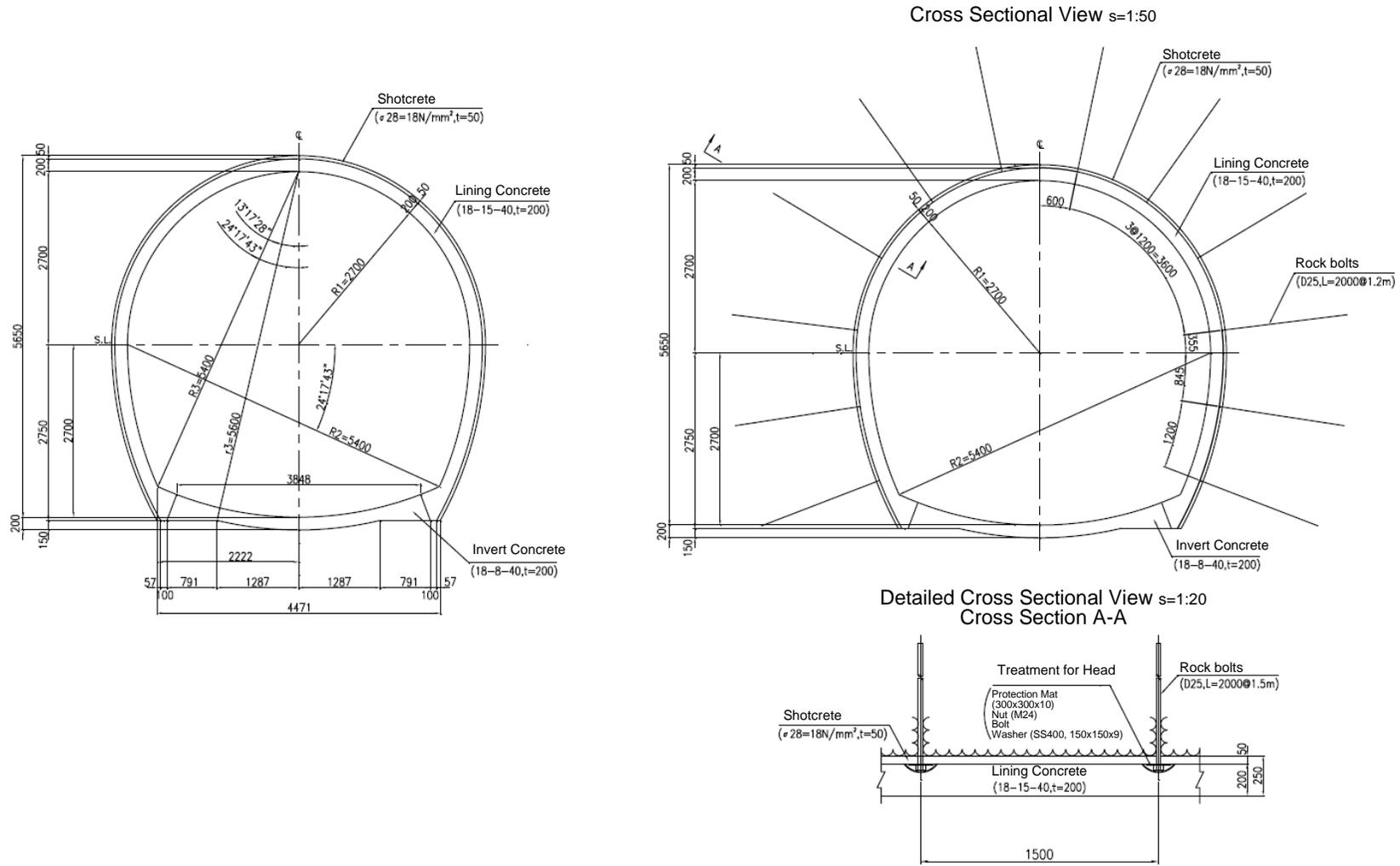
Figure 10.4. Standard cross-sectional view (left) and support pattern (right) of class CI.
