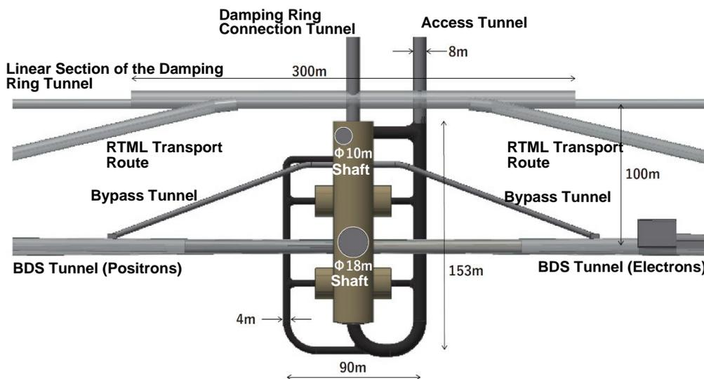
Figure 2.13. Plan view of the periphery of the detector hall.
