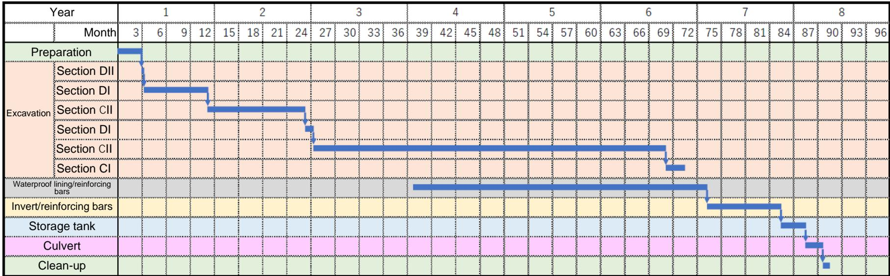
Figure 10.8. Processes for the drainage tunnel.
