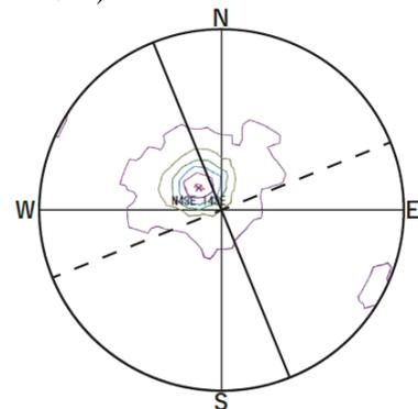
Figure 4.4. Frequency distributions of fissures observed with a borehole camera. The Schmidt net (equal-area projection) is used on a stereonet to express a pole projection chart of a lower hemisphere. Solid lines represent the axial direction of the ILC tunnel, and broken lines represent the main axial direction of the detector hall.
