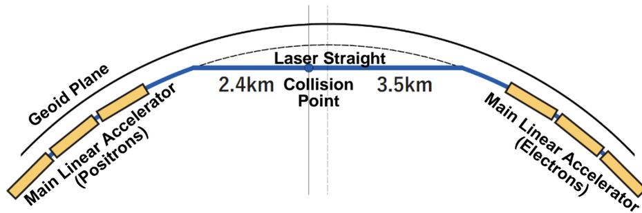
Figure 2.11. Relative position of the ILC accelerator to the geoid plane.
