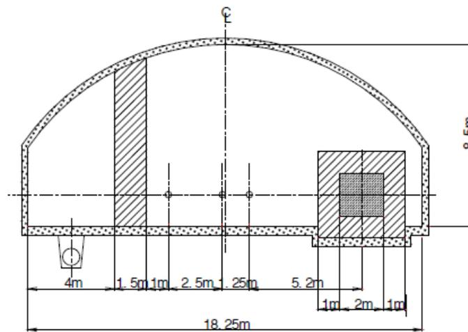
Figure B.5. Cross section C'-C' of the main beam dump cavern.
