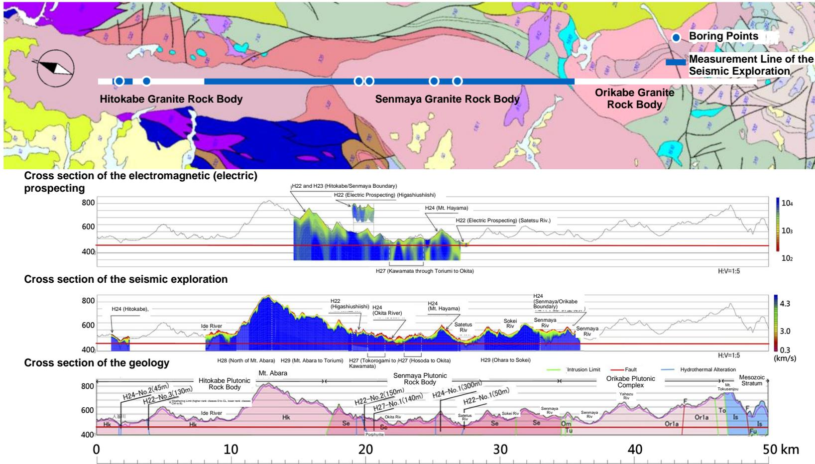
Figure 4.1. Outline of the results of the geological surveys.
