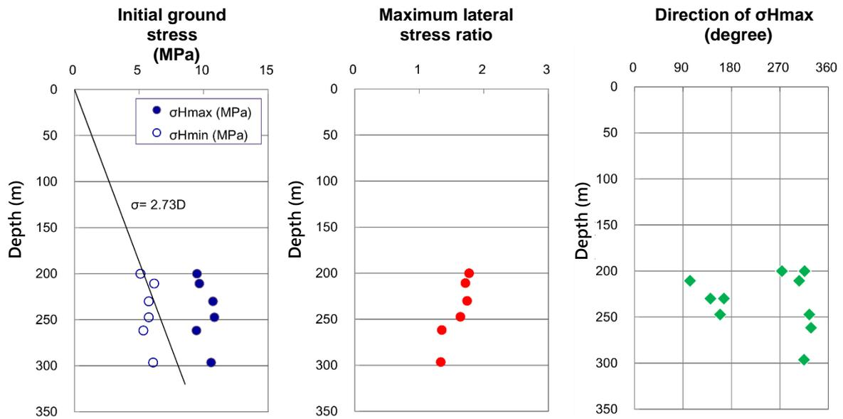
Figure 4.5. Result of the measurement of initial stress.
