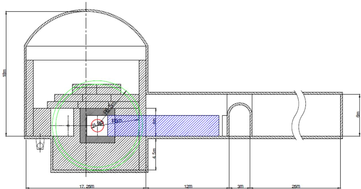
Figure B.3. Cross section B-B of the main beam dump cavern.
