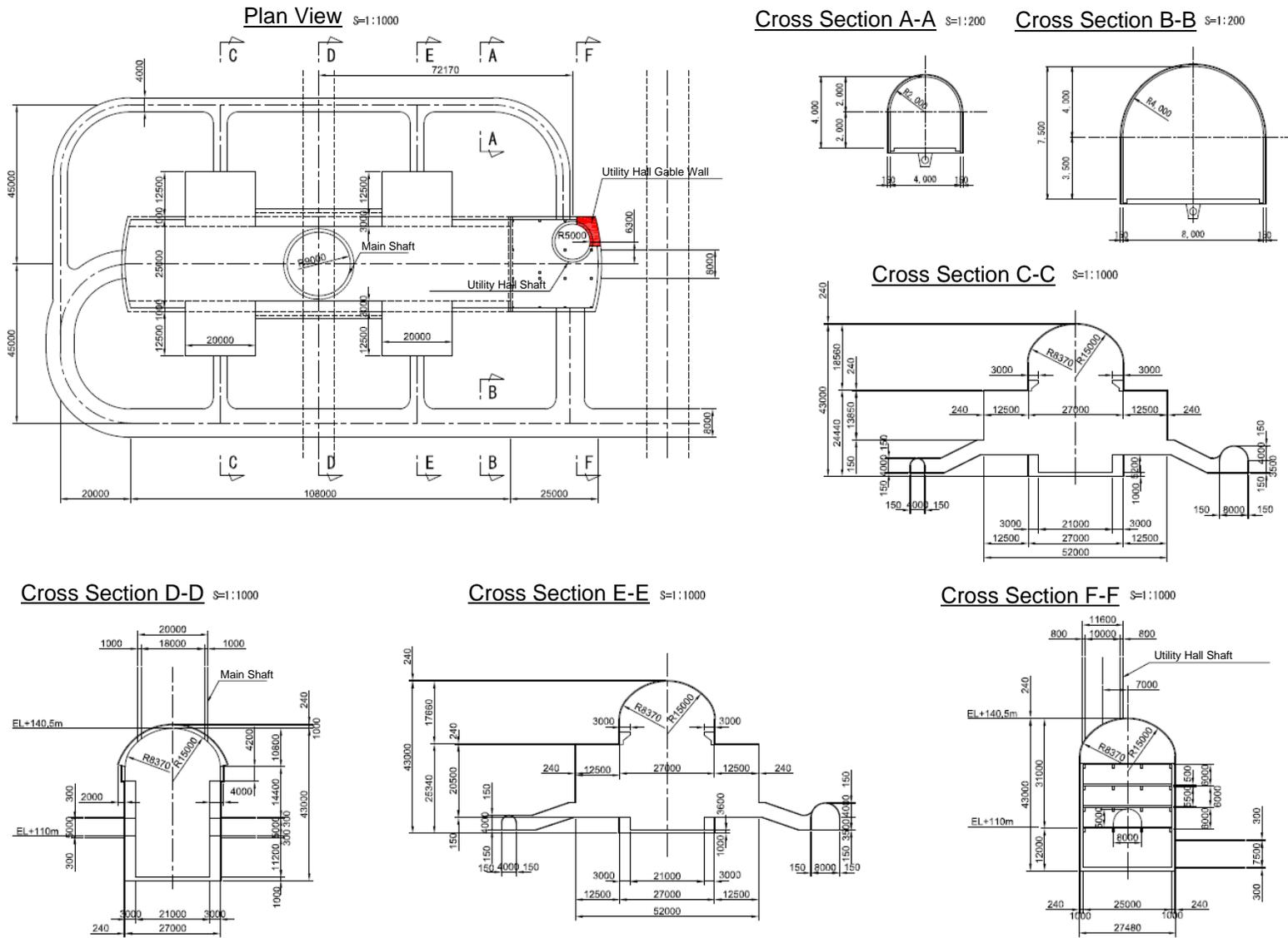
Figure 9.1. A schematic drawing of the detector hall and peripheral tunnels.
