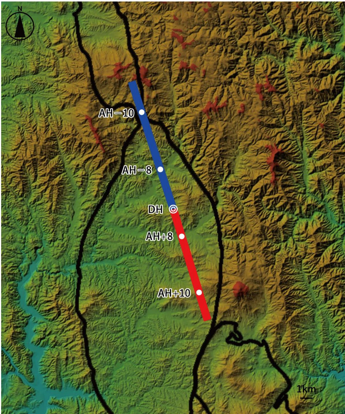
Figure 6.1. A plan view of the topography of the ILC facility location plan (blue line: the main linear accelerator for electrons (a length of 10.9 km), red line: the main linear accelerator for positrons (a length of 9.6 km)).
