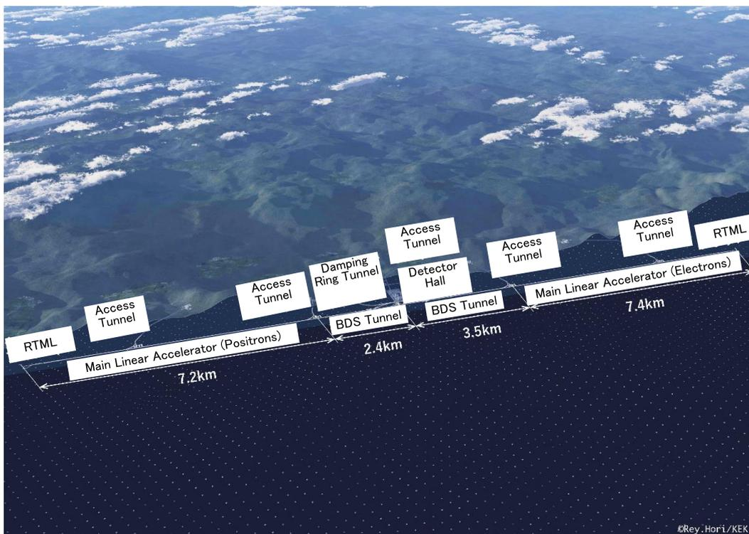
Figure 1.2. Configuration of the ILC underground facility.
