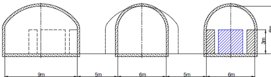
Figure B.6. Cross section D-D of the main beam dump cavern.
