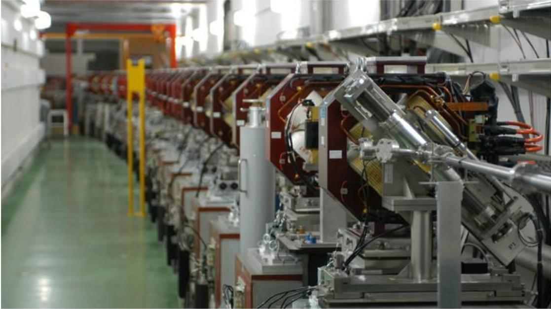
Figure 2.10. ATF2 beamline to demonstrate the BDS technology.
