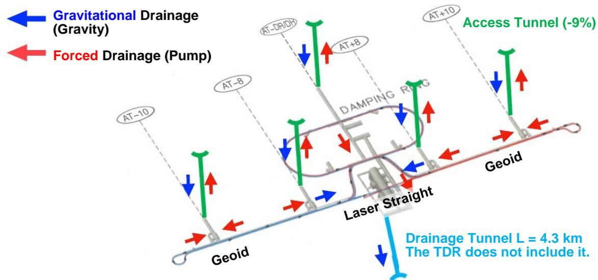
Figure 10.1. A diagram of the drainage system of the underground facility after the beginning of facility usage.
