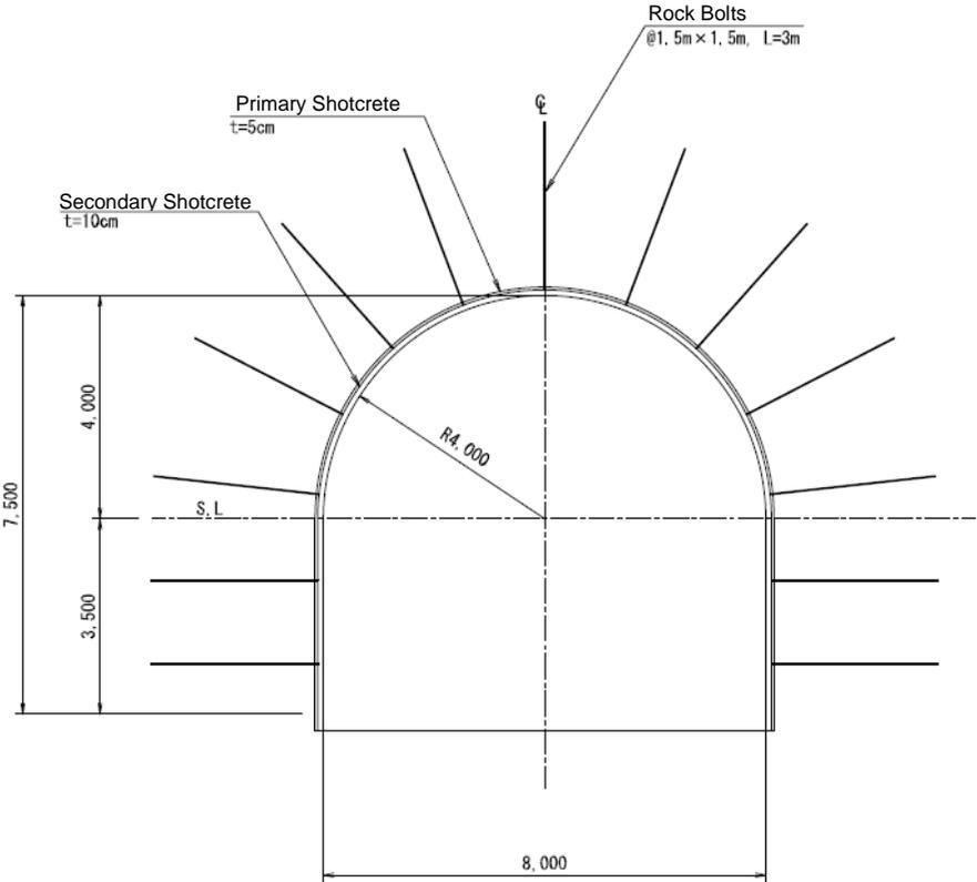
Figure 9.6. Standard support patterns of peripheral tunnels.
