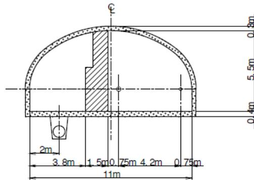
Figure B.2. Cross section A-A of the main beam dump cavern.
