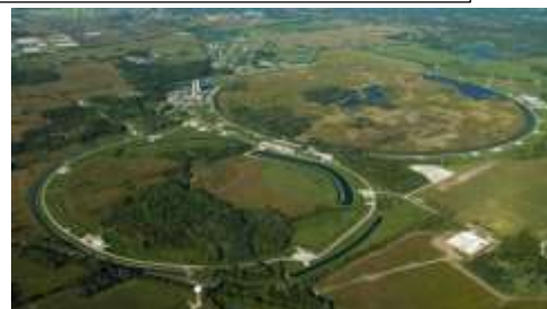
Fermi National Accelerator Laboratory (U.S.) (Circular (6 km in circumference), at approximately 8 m under the ground)
