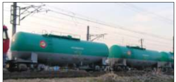
Taki type-1000 freight cars of Japan Freight Railway Company, each of which has an actual capacity of 61.6 m 3
